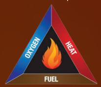
Atmospheric air only consists of 20% oxygen. The rest is Nitrogen (an inert gas), which doesn't burn. We need to take all the Oxygen that is available and ensure that it has the best environment in which to burn.
